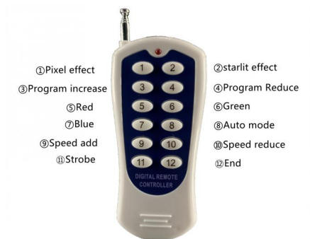
Remote it can shows all on, auto mode, pixel, strobe, more than 40pcs different program
