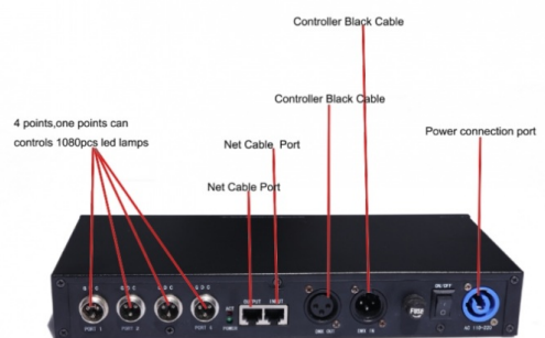
Controller, total 4points one points can control about 1024pcs led
